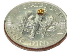
Anaren's new 0606 balun Placed on a dime to demonstrate the significant size reduction and thickness reduction we have achieved with this technology
