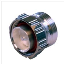
Our adapters come with guaranteed PIM of less than -165dBc @ 2 x 43dBm and are available in any DIN 7/16 or N configuration. Connector savers protect valuable equipment like PIM analyzers and Low PIM loads against port connector wear.
